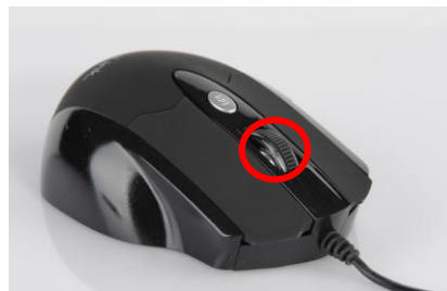
Figure 2. Mouse scrolling button. By sliding the scrolling button of a mouse (highlighted with a red circle in the image), one can navigate through maps or sections within the tool. When placed within the map area, one can use this feature to zoom in and out of specific areas of interest.
